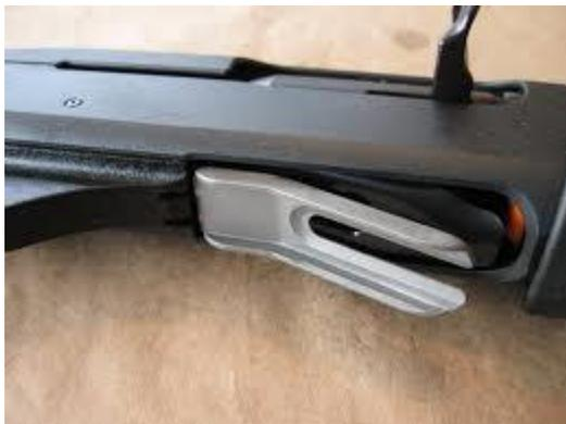
External feed ramp as direct replacement of the carrier release button example (Remington 1100 and 1187 only). Specifically allowed in Standard Div. see point 21.
