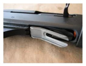
External feed ramp as direct replacement of the carrier release button example (Remington 1100 and 1187 only). Specifically allowed in Standard Div. see point 21.
